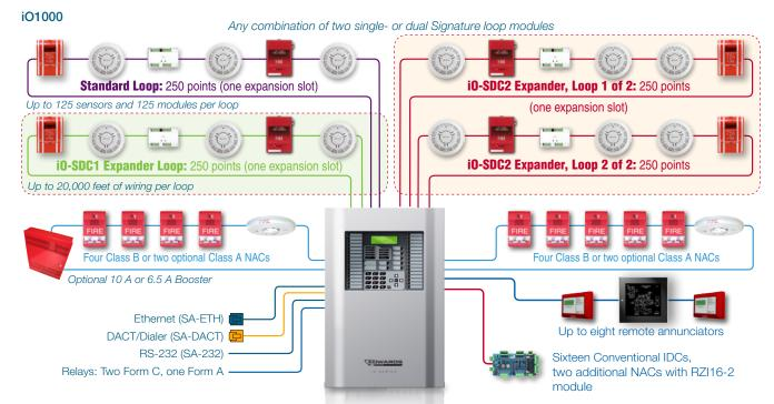
Each iO1000 panel has room for up to two Signature loop controller modules in any combination of single or dual 250-device loops. iO1000 loops support 125 detectors and 125 modules.
